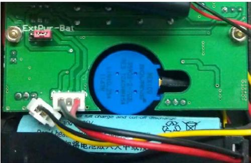
battery will only charge when the AW07A is off. For charging the position of the EXT PWR-BAT jumper does not matter. It will charge in either position.
